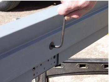
The tool is double-sided; after extensive use some wear may be evident in the threads or face of the tool; simply use the opposite side. Two allen screws and a long-arm allen wrench are also included.
